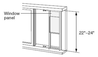
6.5.3 Cut the foam seal (adhesive type) to the proper length attach it on the top of window. Show as below picture.
