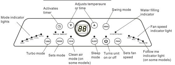
LED display window: Displays setting temperature, Auto timer and malfunction code.
