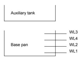
If the water level meets to the WL4, S4 activity, the display will show the P1 protect. All of the loads will into the status of sleep, the unit will back to the origin setting mode unless the water level drops down. The TURBO button is available at P1 protection.
