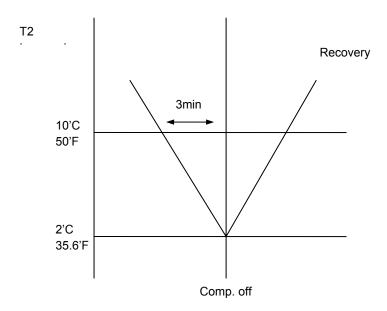
At the anti-freezing control, the pump 1 and pump 2 maintain the origin state. If the mode change to Fan or Heat mode, the time delays safety control cancel. If turn back to cooling mode, timing again.
